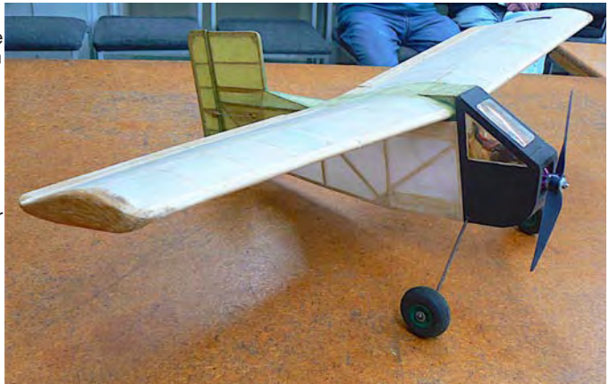
Above: Keith Trillo's IC Tomboy which has a baffle restricting exhaust oil from covering the fuselage.
